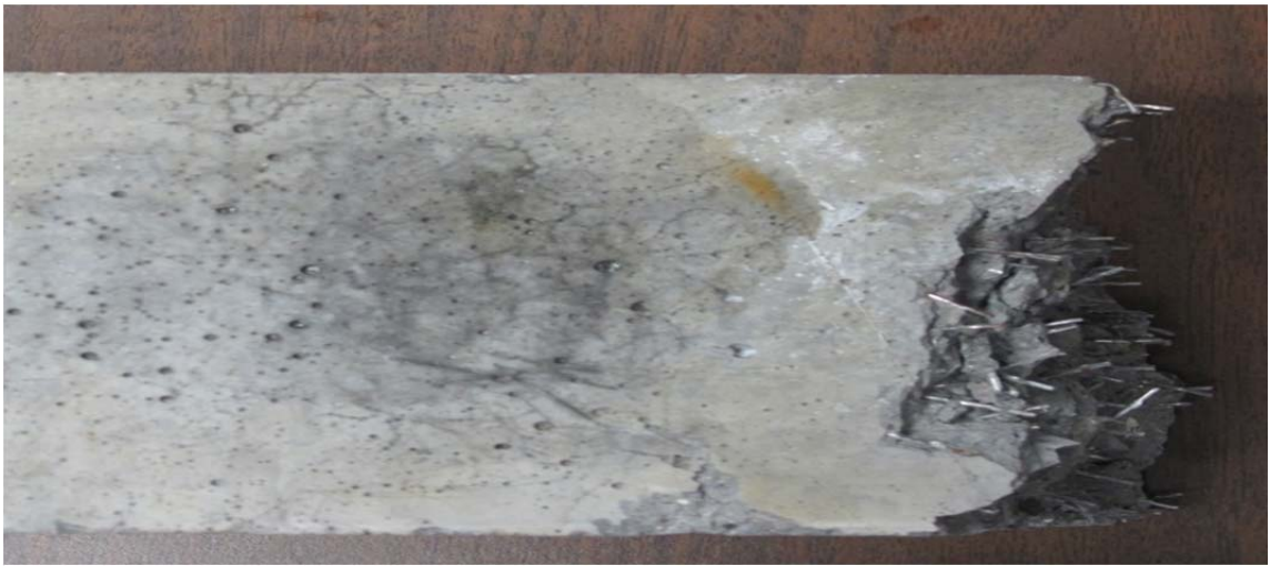
Fig. 5-10: Fiber orientations of a beam sample.
